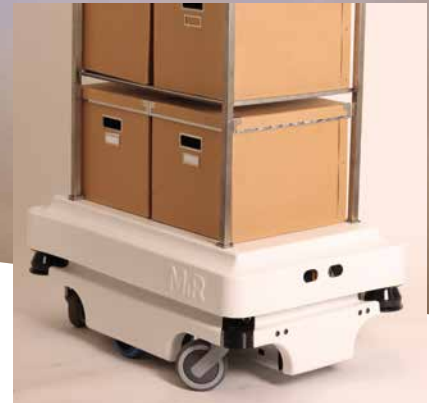
MiR100 can carry up to 100 kg and has the ability to maneuver around moving obstacles.
