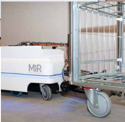
MiR100 is available with a 300 kg capacity tow hook.
