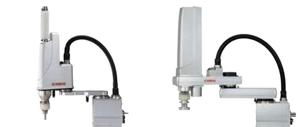
Plays active part in the working environment with a large amount of water or dust (protection class equivalent to IP65).
