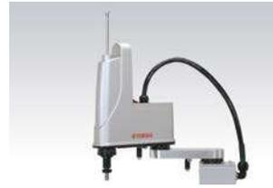
Hollow shaft option convenient for routing of air tubes and harness wires
